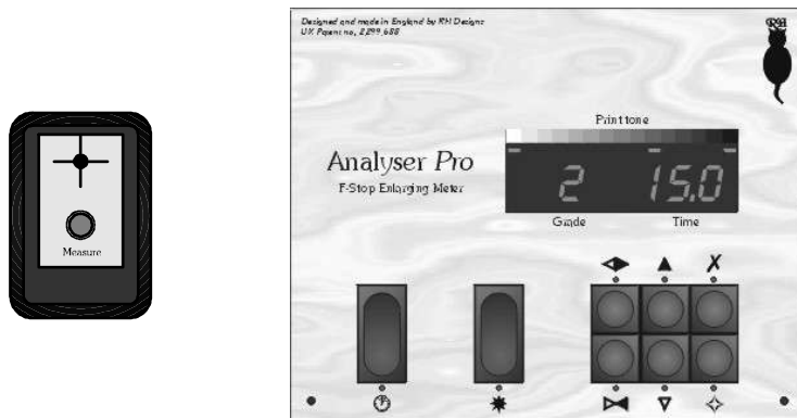
Fig.1. The Remote Sensor and Control Box Front Panel
