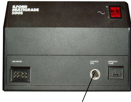
Plug the StopClock 500 into this socket
